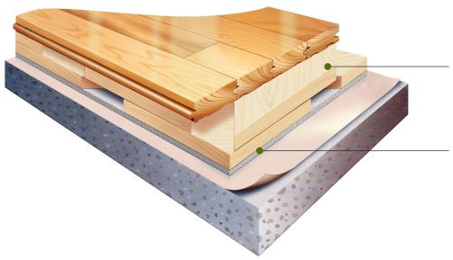
Two Layers 1" x 6" (19 mm x 150 mm) **Subfloor Spacing** (6&2 or 2&2)
