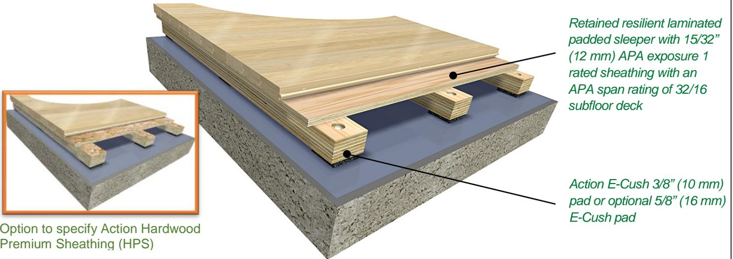
*Retained resilient laminated padded sleeper with 15/32" (12 mm) APA exposure 1 rated sheathing with an APA span rating of 32/16 subfloor deck*
