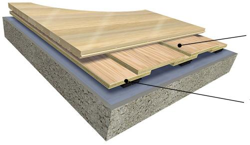
Factory fabricated Double layer plywood subfloor comprised of 15/32" (12 mm) 32/16 span rated
