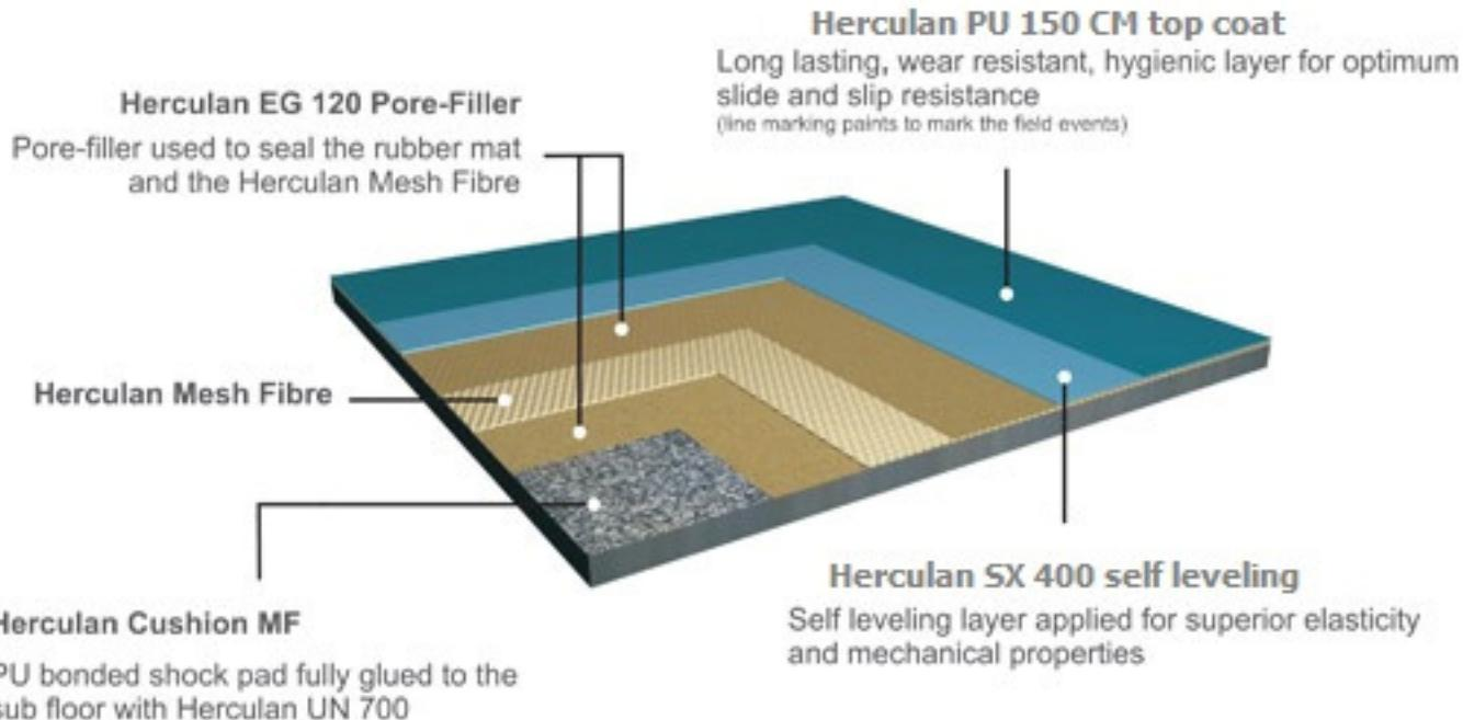
The High performance of the seamless surface of the Action Herculaneum PE Wrestling room floor system is non-porous, hygienic, and easy to clean. The system provides the optimum slide and slip resistance for athletic activities, and its high tensile strength and elasticity of its 2mm urethane surface the system delivers exceptional durability.
