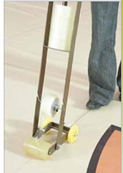
Optional AirRide® tape roller simplifies taping of panel overlaps; tape leaves no residue.
