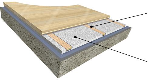
This system's strength comes from its mechanically fastened steel channel with solid wood for flooring fasteners
