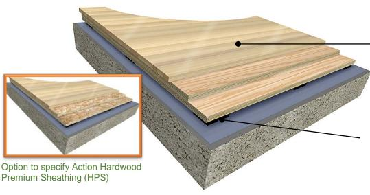
Maple Parquet is adhered directly to multiple layers of 15/23" (12 mm) sheathing subfloor APA rated exposure 1
