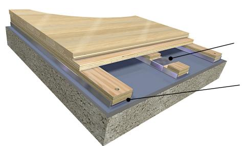
Factory fabricated steel channels and laminated sleepers with resilient pads for exceptional performance and stability.
