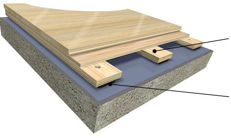
Anchored wide body laminated sleepers and sheathing provide the system with dimensional strength and stability
