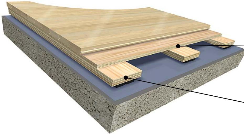
*Wide body laminated sleepers and sheathing provide the system with dimensional strength and stability*
