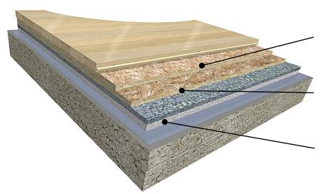
Stable, balanced double layer 15/32" (12 mm) thick, APA exposure 1 rated sheathing minimum APA span rating of 32/16.
